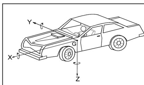
Fig.3 Component coordinate system
