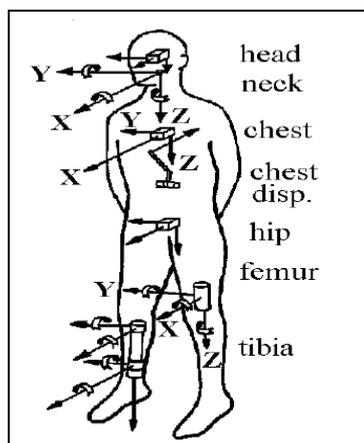
Fig.2 Body coordinate system
