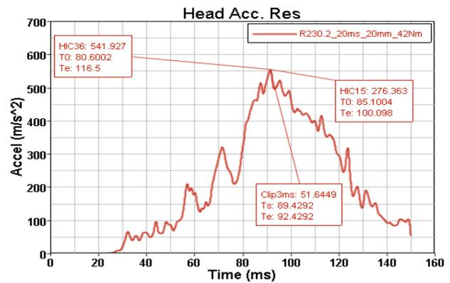
Fig.25 Graph of Head Acceleration V/S Time
